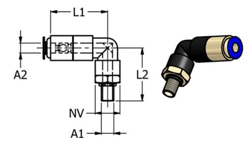
Ext. hose diameter A2 = 6L1 = 29.4 L2 = 21.7 NV = 12 Thread A1 = M5
